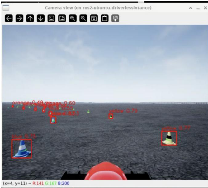
Fig. 4. Camera feed with YOLO bounding boxes. Red rectangles show raw detections; color labels and confidence scores are overlaid. The close blue cone (bottom-left, large bounding box) is correctly verified via stripe brightness; the distant cones (upper frame) rely on YOLO class labels.
