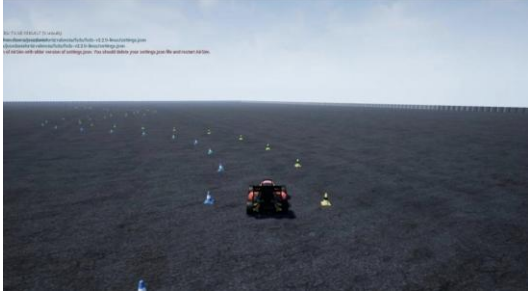
Fig. 2. FSDS simulation environment. The autonomous vehicle navigates a cone-defined track at speed. Blue cones mark the left boundary; yellow cones mark the right. Orange cones mark start/finish and chicane entries.
